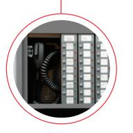
Integrated audio is ideal for emergency communications applications. Up to eight channels of digitized voice allow simultaneous and unique messages to be broadcast to different areas of a facility.
